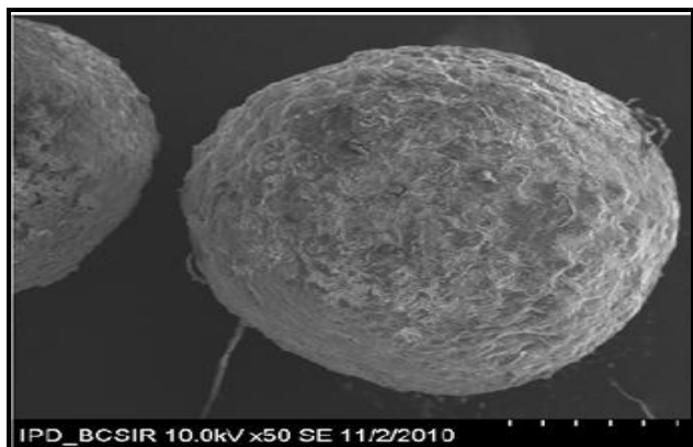
Figure 2: Rough Surface and Spherical Shape of Pellets
