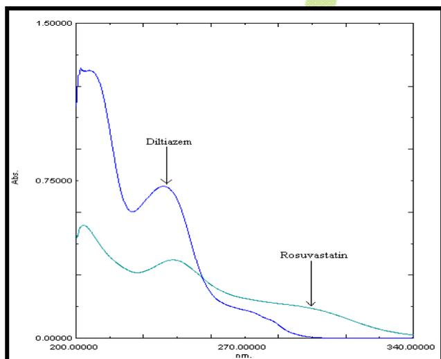
Figure 1: Overlain Zero Order Absorption Spectra of Standard Solution of Rosuvastatin and Diltiazem
