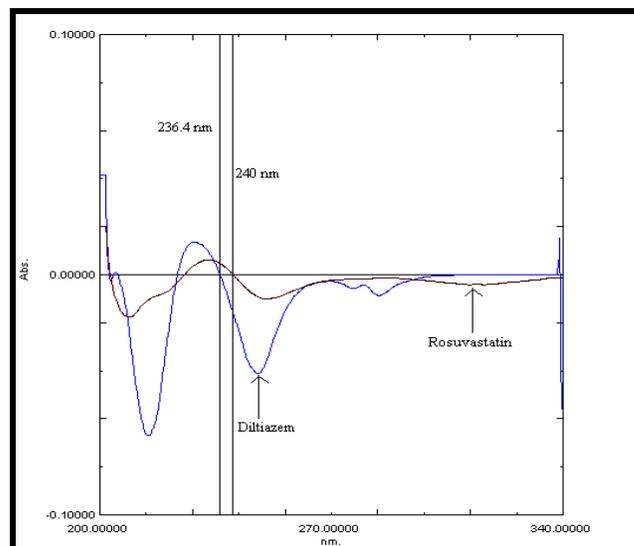
Figure: 2 Overlain First Derivative Absorption Spectra of Standard Solution of Rosuvastatin and Diltiazem
