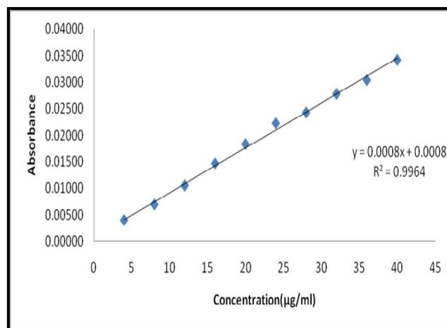
Figure: 3 Calibration Curve of Diltiazem at 240.0nm (ZCP of Rosuvastatin)
