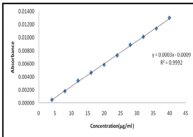
Figure: 4 Calibration Curve of Rosuvastatin at 236.4nm (ZCP of diltiazem)
