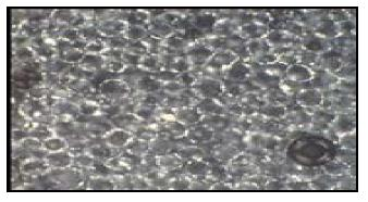
Figure 3: Polarized microscope image of lead emulsion
