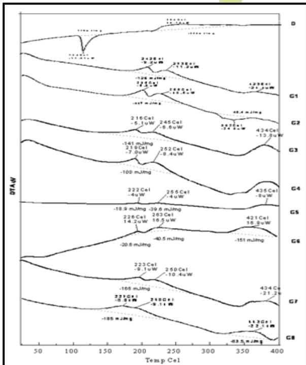
Figure 7(b): DTA curves for BPM drug (D) and drug loaded crosslinked beads (G1-G8)
