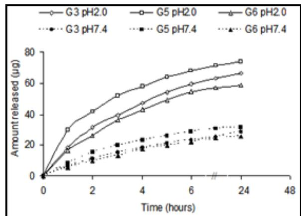
Figure 9(b): Release of BPM from 142 µg BPM loaded bead vs time in solution pH 2.0 and pH 7.4 at 37°C having different weight ratio of chitosan
