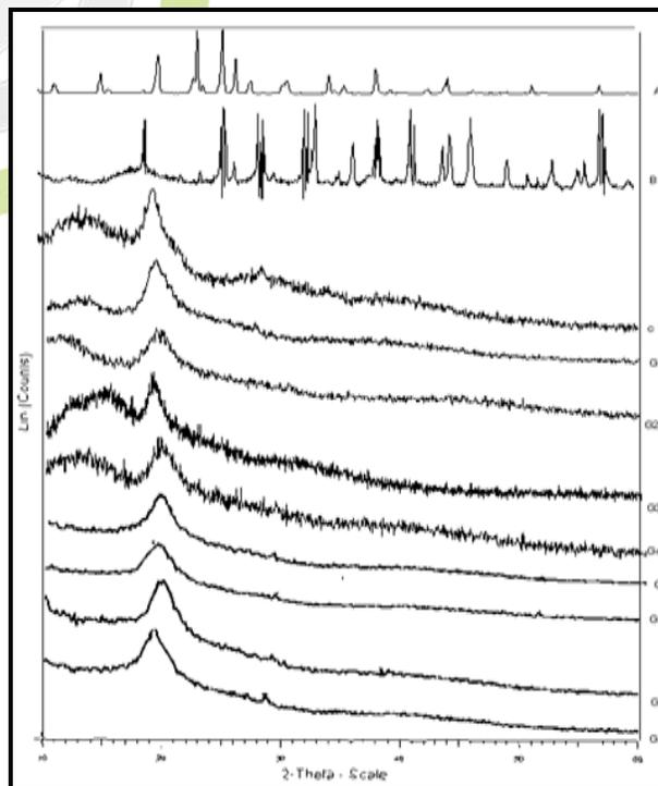
Figure 4(a): XRD graphs of glutamic acid (A), glycine (B), chitosan powder (C) and drug unloaded Cross linked beads (G1-G8)
