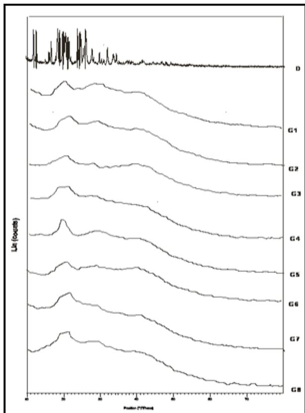
Figure 4(b): XRD graphs of pure BPM drug (D) and drug loaded cross linked beads (G1-G8)
