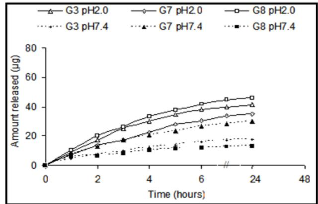
Figure 8(c): Release of BPM from 78 µg BPM loaded beads vs time in solution pH 2.0 and pH 7.4 at 37°C having different weight ratio of amino acid
