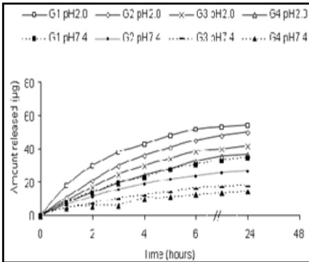
Figure 8(a): Release of BPM from 78 µg BPM loaded beads vs time in solution pH 2.0 and pH 7.4 at 37°C having different percentage of glutaraldehyde
