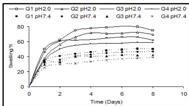
Figure 1(a): Swelling behavior of cross linked beads as a function of time in solution pH 2.0 and pH 7.4 at 37°C having different percentage of glutaraldehyde
