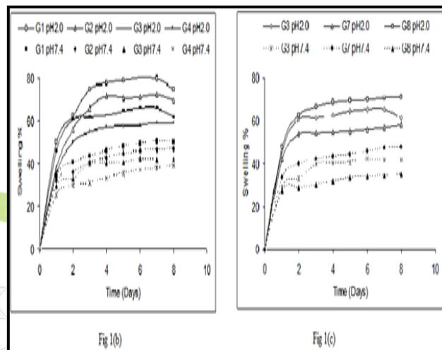
Figure 1(b): Swelling behavior of cross linked beads as a function of time in solution pH 2.0 and pH 7.4 at 37°C having different weight ratio of chitosan
