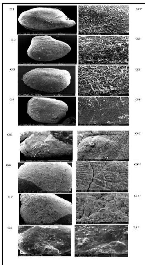
Figure 2: SEM photographs of cross linked beads (G1-G8) and their morphology (G1\*-G8\*)
