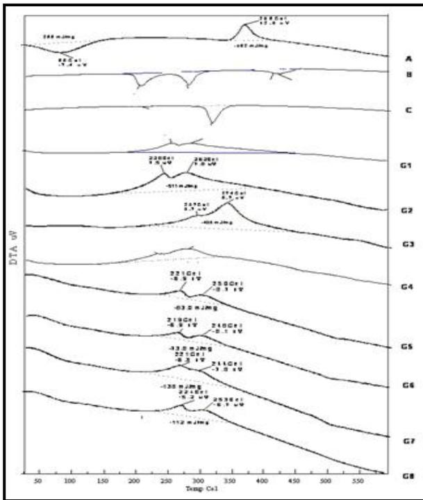
Figure 7(a): DTA curves for chitosan powder (A), glutamic acid (B), glycine (C) and drug unloaded cross linked beads (G1-G8)
