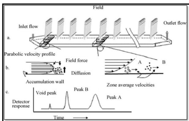
Figure 1: A Schematic Illustration Of The Basic Principle Of Normal Mode FFF Separation And A Typical Resulting Fractogram Are Shown In Fig. 1. The Fractogram Is A Detector Response versus Elution Time (Or Elution Volume)
