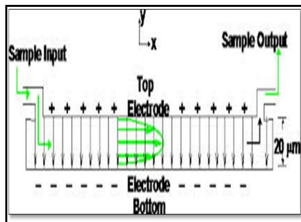
Figure 9: Schematic Representation of EFFF
