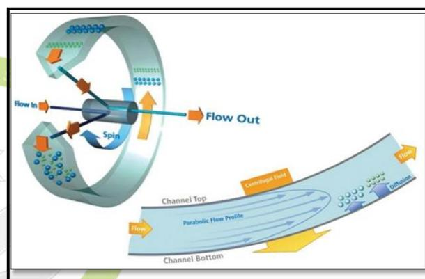
Figure 5: Schematic Representation of SdFFF Instrument
