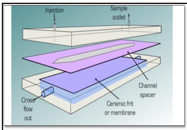
Figure 3: Schematic Representation of Channel of FFF
