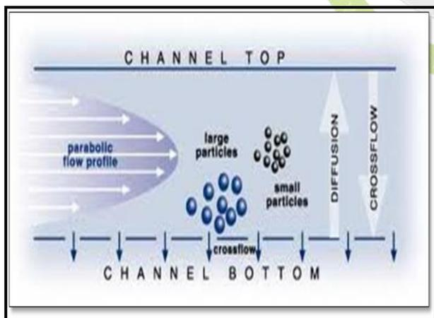
Figure 7: Schematic representation of FIFFF instrument
