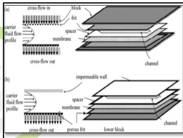
Figure 8: Schematic Representation of (A) Symmetric (FIFFF) and (B) Asymmetric (AsFIFFF) Channel Structures
