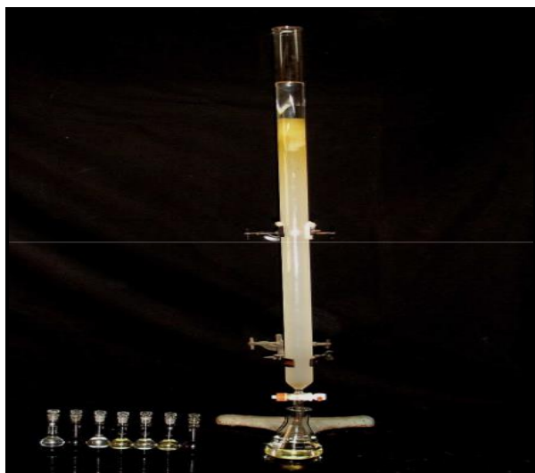
Figure 1: Silica gel column Chromatography
